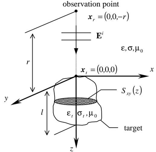
Figure 1: A target embedded in an unbounded homogeneous medium is illuminated by a uniform plane wave.
