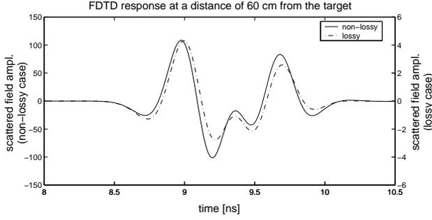
Figure 3: Simulated response of the example target for the non-lossy ( $\epsilon_r = 4, \sigma = 0$ ) and the lossy ( $\epsilon_r = 4, \sigma = 30$  mS/m) host medium.
